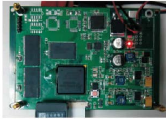
Figure. 4. Lane departure warning system hardware circuit board
